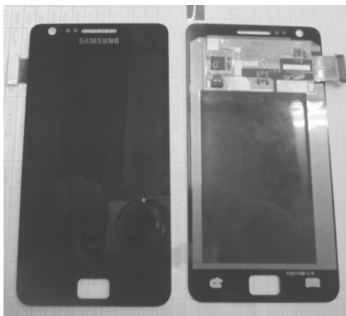
图 5 super AMOLED,对环境光表现出极低的反射 Fig. 5 Extremely low reflectivity of the ambient light, by a super AMOLED module
